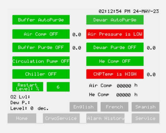
For maintenance. the Maintenance screen supports system purging and technical interventions. enhancing service efficiency. The Initialization screen quides users through setup and purging, automatically transitioning to the Main screen upon completion.
