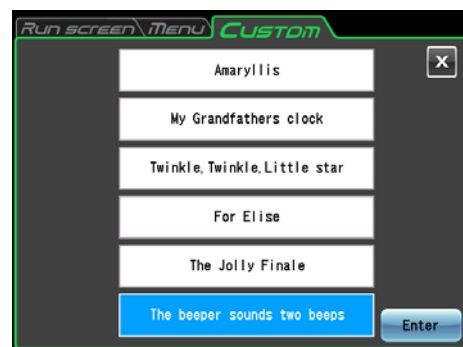
Fig. 3-4-5 (2) Stop signal setting screen
